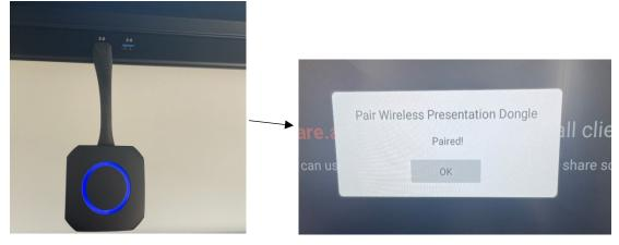
• For your **laptop**: Unplug the Eshare dongle from the Onescreen Touch panel then insert the dongle into your laptop USB port for it to load when finish loading you should see **Tap screen sharing button to start sharing** your laptop.
